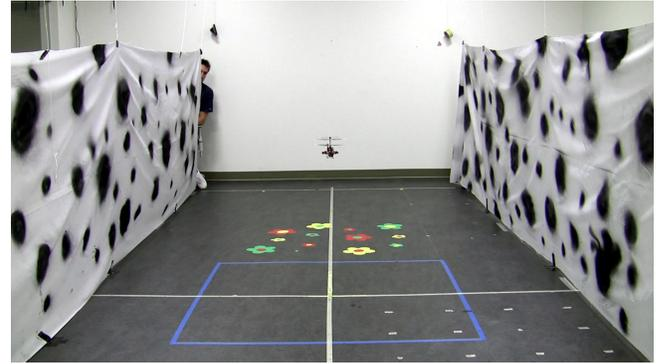
Fig. 5. A photograph of the corridor-like environment within the Vicon arena during an experiment. The dimensions of the corridor were approximately 5.0 m  $\times$  2.6 m  $\times$  1.5 m ( $L \times W \times H$ ).
