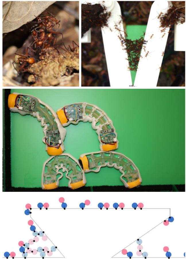
Fig. 1: **Top**: A natural bridge formed by *Eciton hamatum* (Left) and an experimental set-up with the same species (Right, image courtesy of Reid, Lutz, Garnier [4]). **Center**: *Eciton robotica* in a potential ramp structure with two active robots. **Bottom**: Simulated robots form a structure that smooths traffic over rough terrain. Light colors indicate that the agents have gone into a “bridge” state and are stationary.
