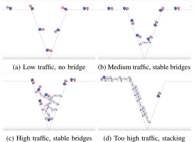
Fig. 7: Bridge formation types, for multiple traffic rates
