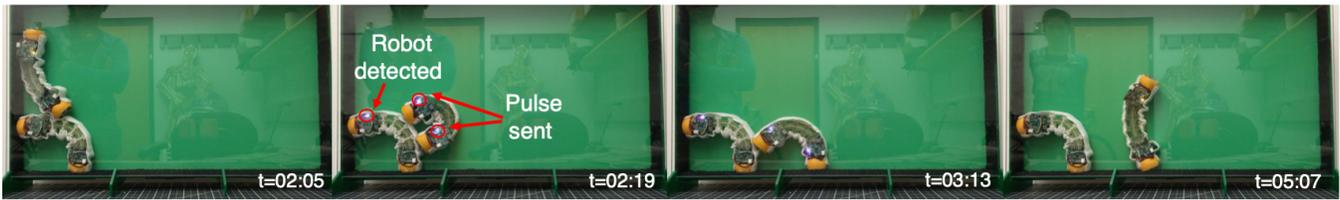
Fig. 3: An *E. robotica* robot climbs over a second robot, which detects its presence as indicated with pink LEDs.
