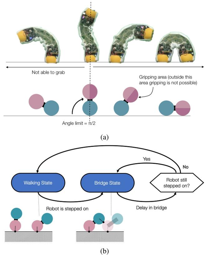
Fig. 5: a) Real robot and simulated robot flip and attach only after going through the neutral position. b) State machine for a simulated robot consists of two states: (i) the walking state where the robot continuously flips and moves forward, and (ii) the bridge state where the robot remains stationary as a result of sensing being stepped over.
