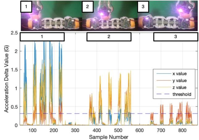
Fig. 4: Vibration pulse detection: A graph of the change in acceleration (delta) values for the detecting robot. Measurements are taken from bottom robot on the left side PCB; a vibration pulse is sent from a gripper attached at (1) the close end (2) the center and (3) the far end of the robot. Using the chosen threshold, the robot can detect pulses at any point along its body.
