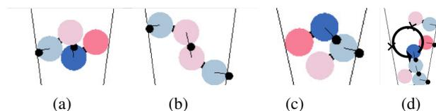
Fig. 10: Bridge dissolution failures: (a) A bridge robot grabbed from below (b) Two bridge robots grabbing each other (c) Walking (top) robot stuck in the terrain (d) Trapped walking robot which moves in circles
