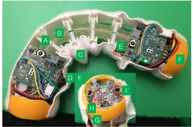
Fig. 2: An *Ecton robotica* agent. The body is composed of rigid (A) and flexible (B) portions, and is covered in stretchy Velcro loop (C). A motor and spool (D) winds a cable (E) on both the top and bottom to control the bending of the robot. Grippers (F) on each end attach to velcro surfaces. A motor (G) on each gripper controls the four corkscrews (H) to attach which wind into the velcro. Two IR sensors (I) detect when a gripper has made contact with a new surface.
